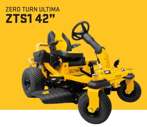
Model Number:MT17BAGBYE330Engine:679cc Cub Cadet EngineDrive System:Dual Hydro-Gear EZT 2200
